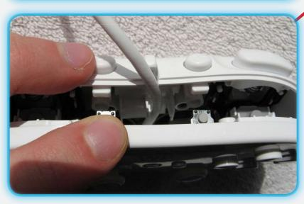
10: Close up the controller and run the wire through the openings that you have created. You can use the shaft of a screwdriver to push the wire into the gap, as indicated by the arrow. Then use the tri-wing for the last five screws on the backside. Tighten them firmly.
